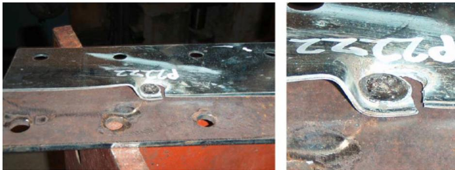
Figure 1.4: Sheet tearing failure mode (Guenfoud, 2010).
