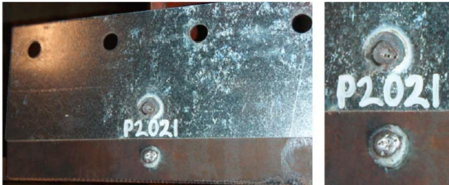
Figure 1.3: Shear weld failure (Guenfoud, 2010).
