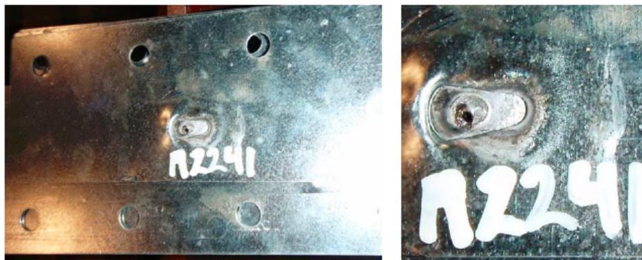
Figure 1.5: Sheet bearing failure mode (Guenfoud, 2010).
