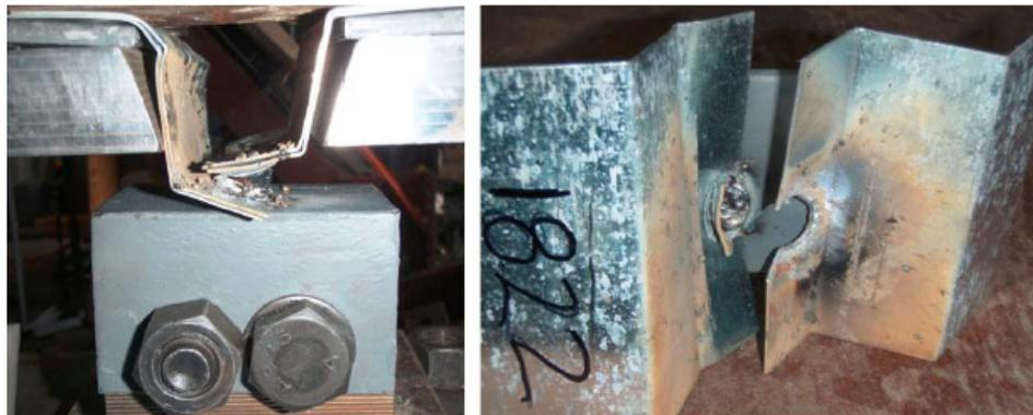
Figure 1.7: Tension sheet failure (Guenfoud, 2010).
