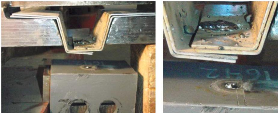
Figure 1.6: Tension weld failure (Guenfoud, 2010).
