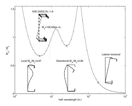
Figure 2 Buckling Modes for a C-section
