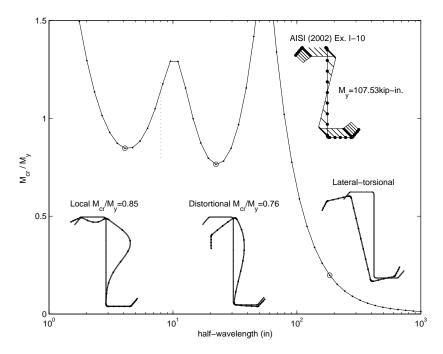
Figure 1 Buckling Modes for a Z-section
