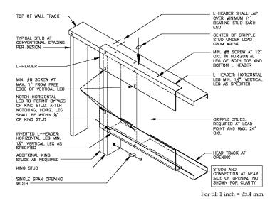
Figure 5: Inverted L-Header Assembly
