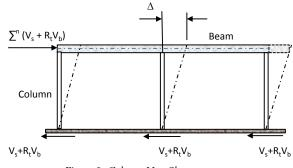
Figure 3: Column Vase Shear.
