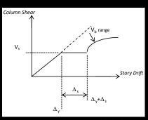
Figure 2: Structural Response of Bolted Connection.
