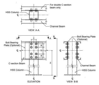
Figure 2: Typical CFS-SBMF Moment Connection.
