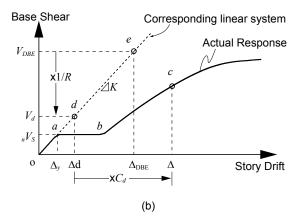
Figure 7: CBF-SBMF Expected Response: (a) Yield Mechanism and Column Shear Distribution; (b) General Structural Response.
