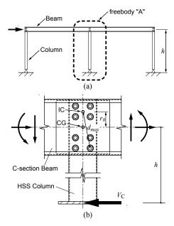
*Figure 5: Bolt Group in Eccentric Shear: (a) CFS-SBMF; (b) Freebody "A".*
