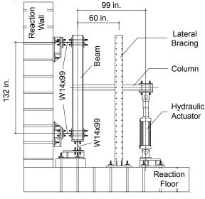
Figure 3: Test Setup.
